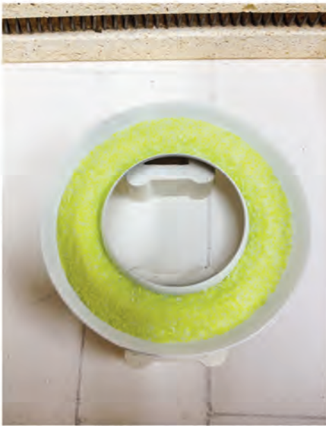
Elevate the mold approx. 1 ½" in the kiln.
