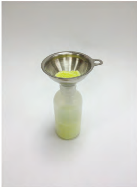
Transfer the mixed frit into a squeeze bottle. A small funnel makes this task a little easier.
