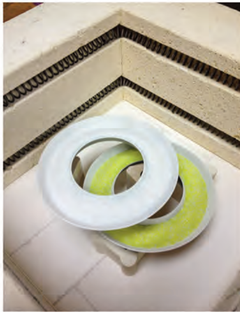
Option: The size and design of the bangle bracelet mold allows you to cast two bracelets comfortably in an 8" table-top kiln. Prepare and fill a second mold and elevate approx. 2 ½".
