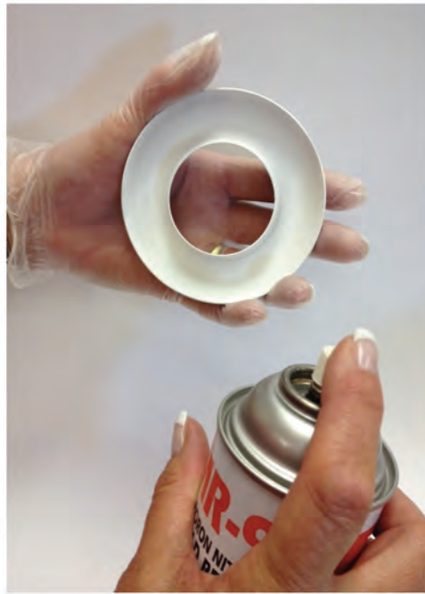
Prepare the bangle bracelet mold. For this project I am preparing the mold with MR-97.
